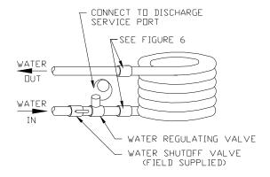
FIGURE 5 - TYPICAL CONDENSER WATER PIPING
